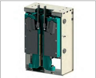
Braking force generated through a combination of disc springs and braking elements (adjustable by the disc spring assembly) activated. Simple and compact design for easy integration in different positions on car slings or counterweight frames. Low force needed to release after engagement.
